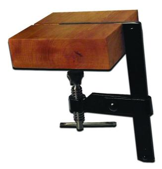
Universal clamp used mainly for fixed mounting of locksmith vices on workbench top without board destruction or drilling. Thanks to its rigidity and stable construction it is very firmly fixed, easy and quick installation and removal due to trapezoidal screw thread. The clamp dimensions are  $260 \times 200 \times 170 \, \text{mm}$ , maximum of  $160 \, \text{mm}$ .
